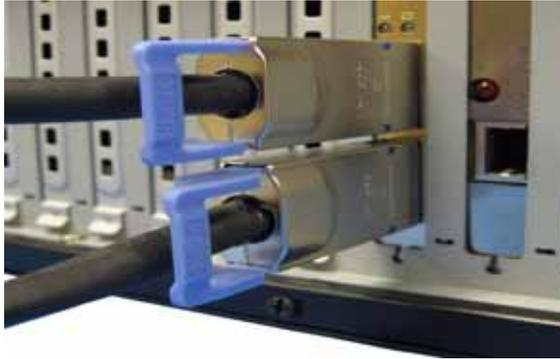
9. Connect at least one cable from the DXE410 chassis to the DXH510 host adapter. The cable should be connected with the corresponding ports connected to each other. For examples, connect the cable from port P0 on the DXE410 to P0 on the DXH510.
