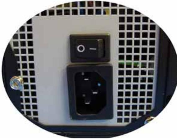
*The front power switch is not a disconnect switch for system power.*
