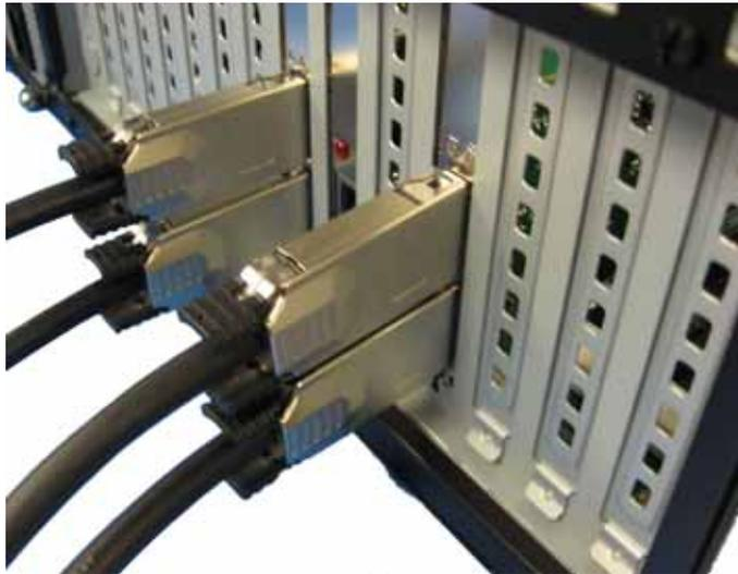
8. Connect one cable for a x4 connection or two cables for a x8 connection from each DXU405 Uplink card to each DXH510 host adapter. The cable should be connected with the corresponding ports connected to each other. For examples, connect the cable from port P0 on the DXU405 uplink card to P0 on the DXH510 host adapter.
