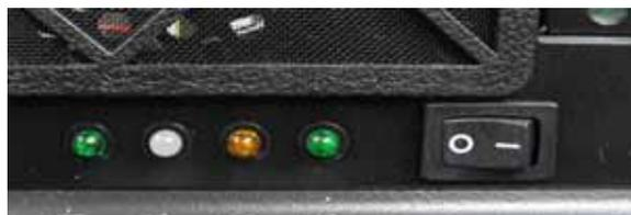
**Note:** *The front power switch is not a power disconnect switch. If installing new peripheral cards or servicing the chassis, be sure to remove the power cord.*
