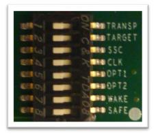
The DIP switch on the PXH812 is used to configure the adapter card. Please leave all undocumented DIP switches in the default position.
