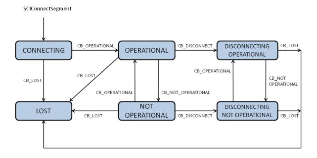
Figure 2: State diagram for a remote segment
